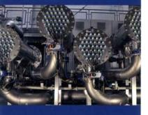
There are no economic ways of removing nitrosamines from water using known water treatment processes. PWT Wasser- und Abwassertechnik GmbH has therefore developed a new process for removing these substances from water using UV technology; tests under practice conditions have proved successful. PWT's UV plants are 100 % made from stainless steel. The plants are fully automated and fitted with equipment for the continuous monitoring of its operation.
